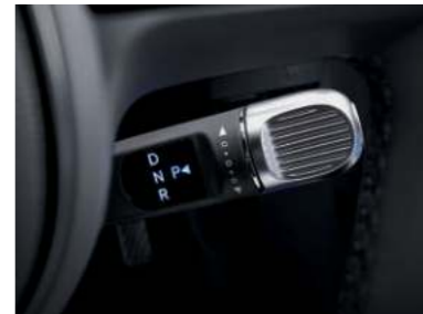
Column rotatory type Shift-by-Wire
