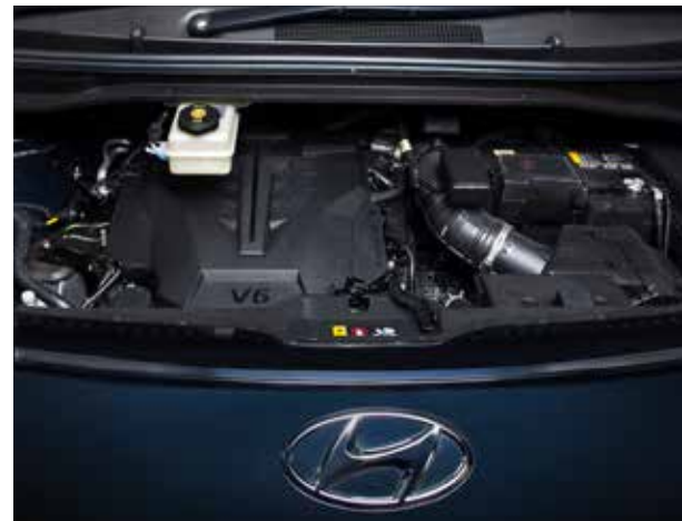
V6 λ III 3.5 MPI engine
