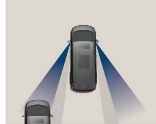
Blind-Spot View Monitor (BVM) When operating the turn signal switch, BVM displays video of the blind-spot view for the direction indicated.
