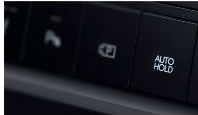
Auto Brake Hold The addition of this function helps add another layer to the vehicle's safety as it prevents the vehicle from rolling off a slope unexpectedly.
