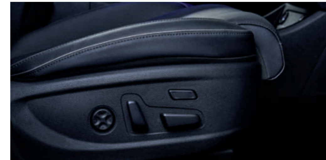
10-Way Power Adjustment + Driver 4-way Lumbar Support
